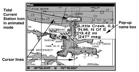
Navionics chart showing Tidal Current Station icon selected by cursor. In this example, the tidal current is in flood but it's about to enter the slack water stage. The current is flowing to the west at 0.1 mph.
